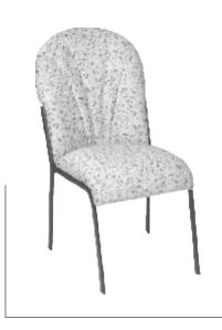
**SPECIFICATION:** Frame work of CRC (Cold Rolled Carbon) Steel pipe 3/4" or  $1\frac{1}{4}$ " flat, 16 gauge wall thickness, electric/gas welded and duly Epoxy powder coated in desired shade. Seat and back frame of solid 1/2" moulded ply wood. 45mm thick, 40 density U Foam in seat and 25 mm thick 23 density U Foam in back with upholstery upto Rs. 100/- per meter with nylon shoes and stacking bushes.
